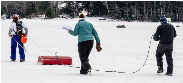
Fig. 2 Ground Penetrating Radar in Action
