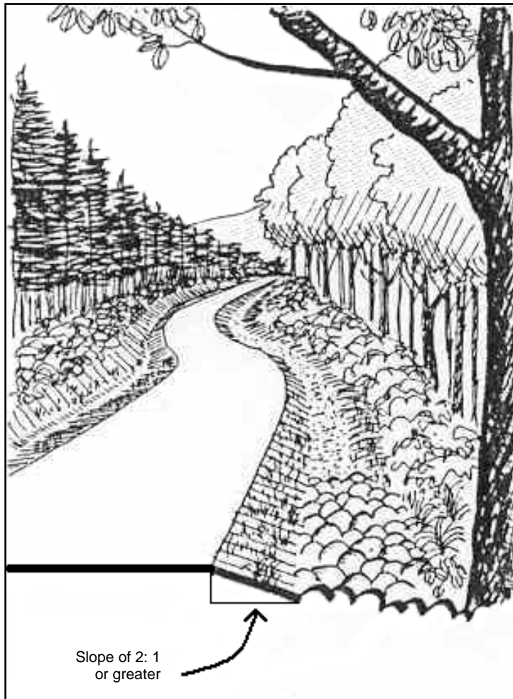
Roadside ditch draining to a rock diffuser set at least 50' from the water.
